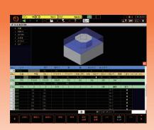
A 3D rendering is created based on the input from the MAZATROL unit in real time
