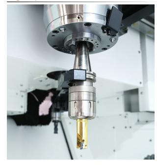
Our high-speed ATC system employs a simple and reliable servo-driven cam actuation system that aids in rapid tool change to reduce non-cut time. Spindle utilization is also increased through bi-directional rotation of the magazine to the next required tool position offering enhanced productivity.
