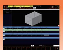
Create a stock unit to define the size of the material and orientation in the machine
