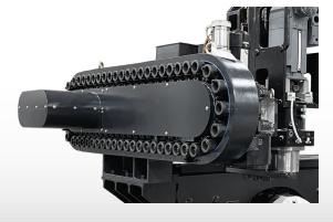
High-capacity CAT 40 tool magazines, common throughout the Ez Series, minimize setups for a variety of workpieces while ensuring adequate tooling for uninterrupted operation.
