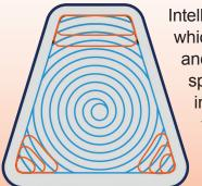
Intelligent Pocket Milling is a MAZATROL pocket machining cycle which calculates a constant contact angle between the tool edge and the workpiece material. This intelligent path controls spindle and axis fluctuations, extending tool life and improving machining efficiency especially in difficult-to-machine materials.
